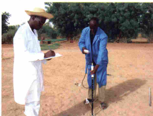
Soil moisture measurement with TDR probe
