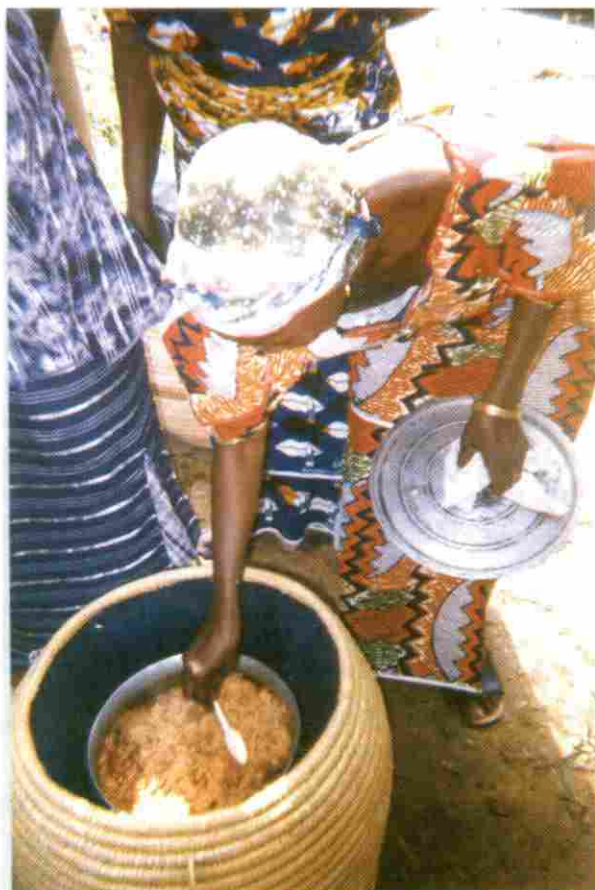
The BITATORE is an efficient energy saving cooking device specially developed for the Sahelian communities
