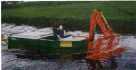
Cutter boat with front loader and a two-screw engine
