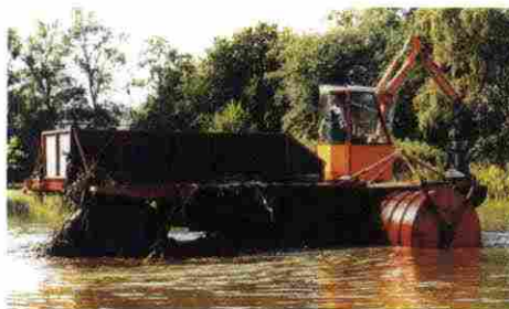
Amphibious vehicle with balloon tyres and floating
