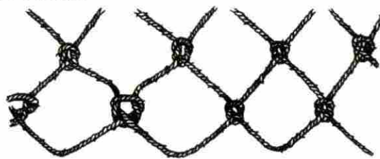
Nets made of twisted fibres
