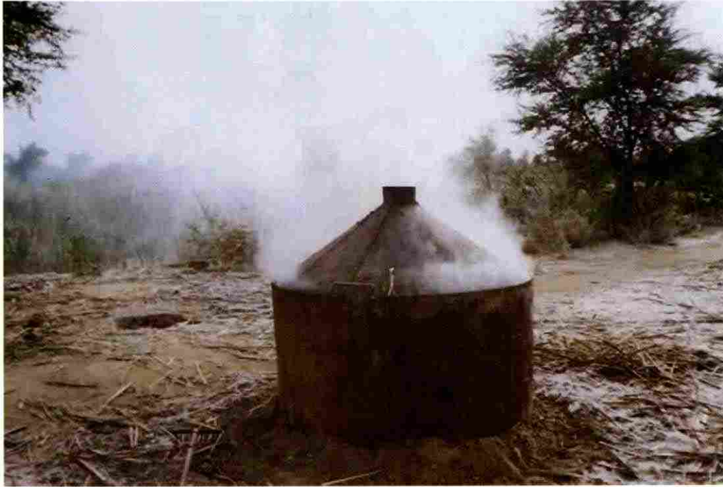
The "3-drum" carboniser in action
