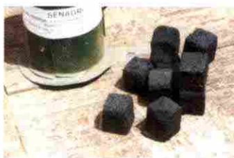
Cubic briquettes made by adding molasses
