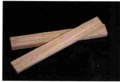
Typha construction timber (bonded stems)
